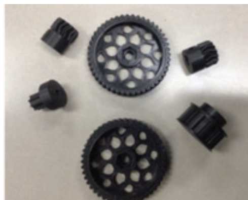
Gears designed in Tinkercad software and 3D printed by students
