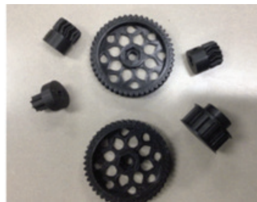
Gears designed in Tinkercad software and 3D printed by students
